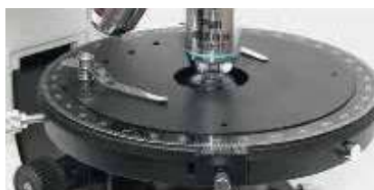
Center-adjustable and turnable polarisation stage
