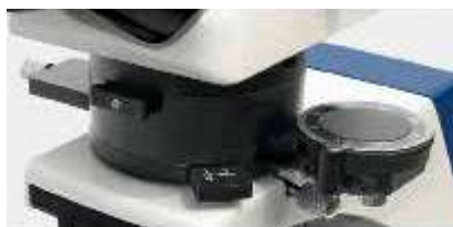
Bertrand lens, λ Slip, 360° rotatable analyser (removable)
