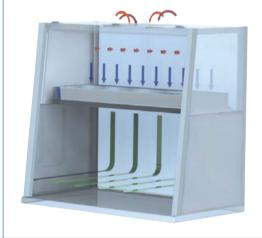
Vertical Air Flow of "MaXtream V"
