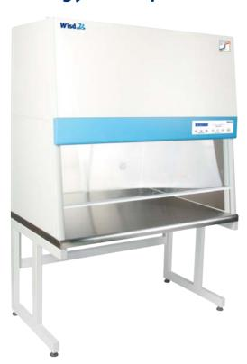
The newly developed Laminar Flow Clean Bench from DAIHAN Scientific provides reliable protection for samples and work processes against particulate contamination. The air from above the cabinet vertically goes through a **Pre-filter and a Class 100 HEPA Filter** of efficiency up to 99.97% & 0.3 micron size and is exhausted to the front opening for maintenance of Contamination-Free in the cabinet. Also **UV Lamp** installed in the cabinet contributes to sterilize a source of contamination.
