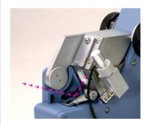
Close the shutter on the upper prism and lower the mirror shutter on the lower prism. This will allow light to be reflected off of the underside of the sample.
