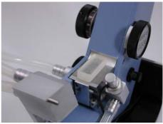
It is important to use the correct amount of contact liquid; there should be just sufficient to cover the interface but should not spread beyond the test piece edges. The correct amount can only be found with experience.
