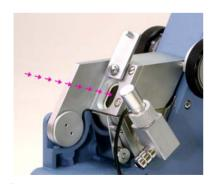
Open the shutter on the upper prism and raise the mirror shutter on the lower prism. This will allow light to pass through the upper prism and the sample.
