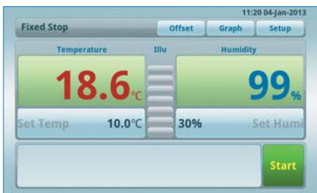
7" Full Touch Screen TFT LCD (Smart-Lab™ Controller)
